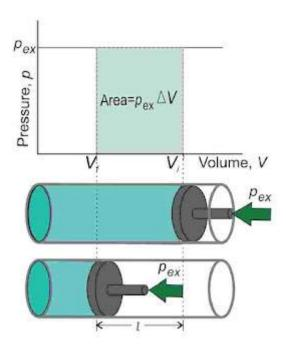
Let the external pressure acting on the piston is Pex. If the external pressure Pex is slightly greater than P piston moves downward till the pressure inside the cylinder becomes equal to Pex. Let this change be achieved in a single step and the final volume be Vf. During this
